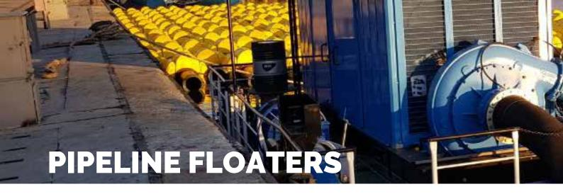
Pipeline floaters – a pipeline, used to transport slurry (a mixture of water and soil or rock, obtained by excavating and mining hydraulically) with hydraulic dredger equipment to the point of discharge.
